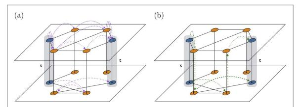
**Figure 1.** Shortest paths in multiplex networks. An element traveling between locations s and t on the multiplex structure has to choose a path among the possible ones shown in the figure. There are 6 shortest paths between s and t, all of them of length 3. Purple lines in panel (a) show classical single layer shortest paths, laying within a unique layer. Green lines in panel (b) show multiplex shortest paths, which make use of interlayer links to jump between layers.
