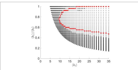
**Figure 4.** Estimation of the congestion induced by the multiplex structure. Light grey region corresponds to configurations where the multiplex induces congestion, and dark grey to regions where the multiplex structure does not induce congestion. Red line represents our semi-analytical estimation of the frontier between these two regions, using (21) and (22).
