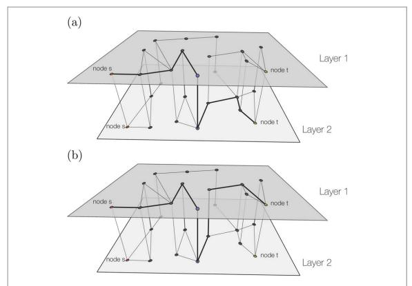
Figure 2. (a) Shortest path in the multiplex network containing a single interlayer link. (b) Shortest path in the multiplex network including two interlayer links.
