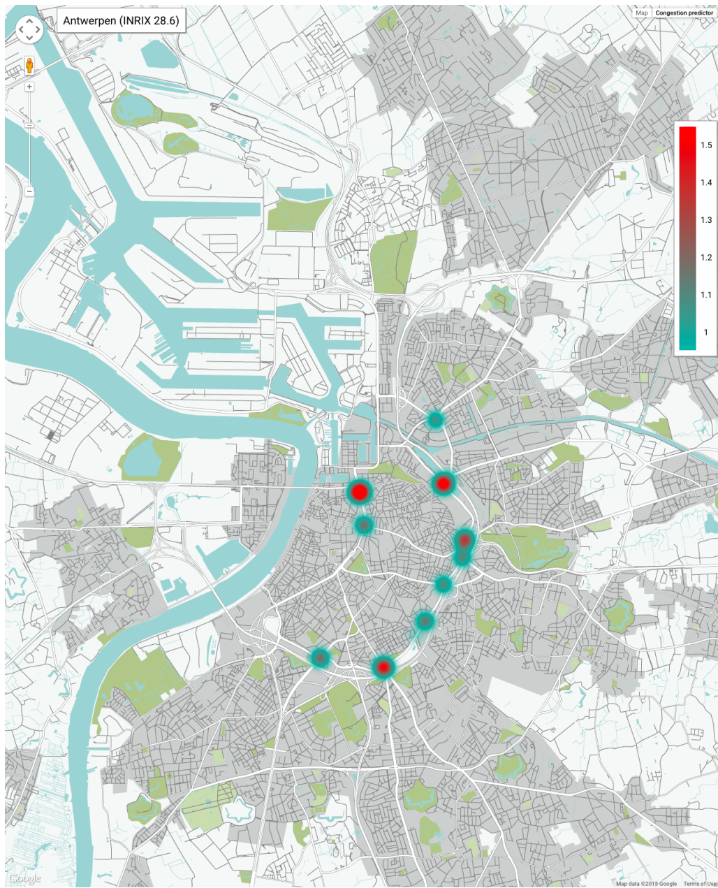
Supplementary Figure 10: Map of Antwerpen showing the expected ratio between incoming and outgoing vehicles of each congested junction, (\sigma_i + g_i)/d_i . Several congested junctions might appear merged in the heat map. Model parameters have been obtained assuming homogeneously distributed source and destination locations and the required road traffic to obtain an order parameter \eta [1, 2] equivalent to the city INRIX value.
