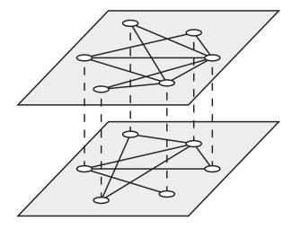
FIG. 1. Example of a multiplex network with M=2 layers. Nodes are the same in both layers. The connectivity at each layer is independent of each other, and the connectivity interlayer is from each node to itself (dashed links).
