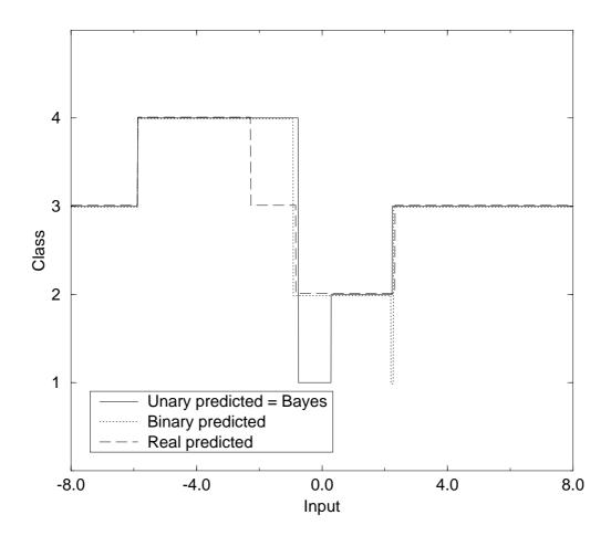
Figure 4: Predicted classifications for the four gaussians problem. Only the unary output representation achieves the desired Bayes classification, whereas both binary and real representations give the wrong answer for certain values of the inputs.
