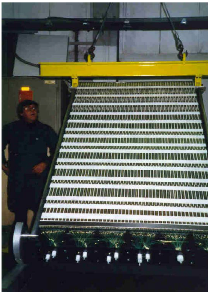
Figure 5.20: One of the first HCAL prototype modules after optics assembly.
