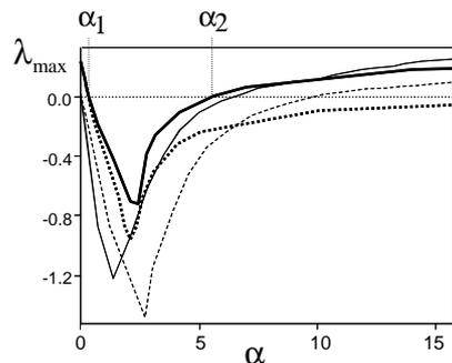
FIG. 8 Four master stability functions for coupled Rössler oscillators: chaotic (bold) and periodic (regular lines); with  $y$  coupling (dashed) and  $x$  coupling (solid lines). (The curves are scaled for clearer visualization). From Barahona and Pecora (2002).
